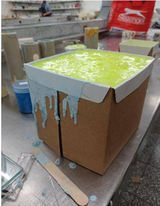
**Figure 5.** (Left) Image taken by April Lannigan; documenting a wet Remade pour into cardboard cast, Midton(2022)
